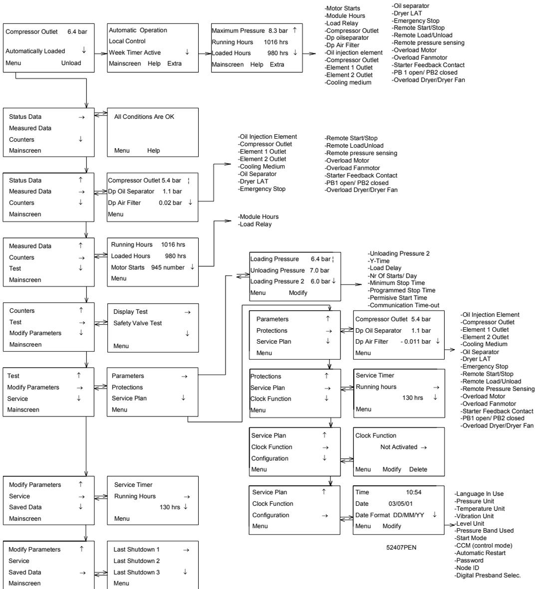
Fig. 4.1 Menu flow, GA90/315 aircooled
