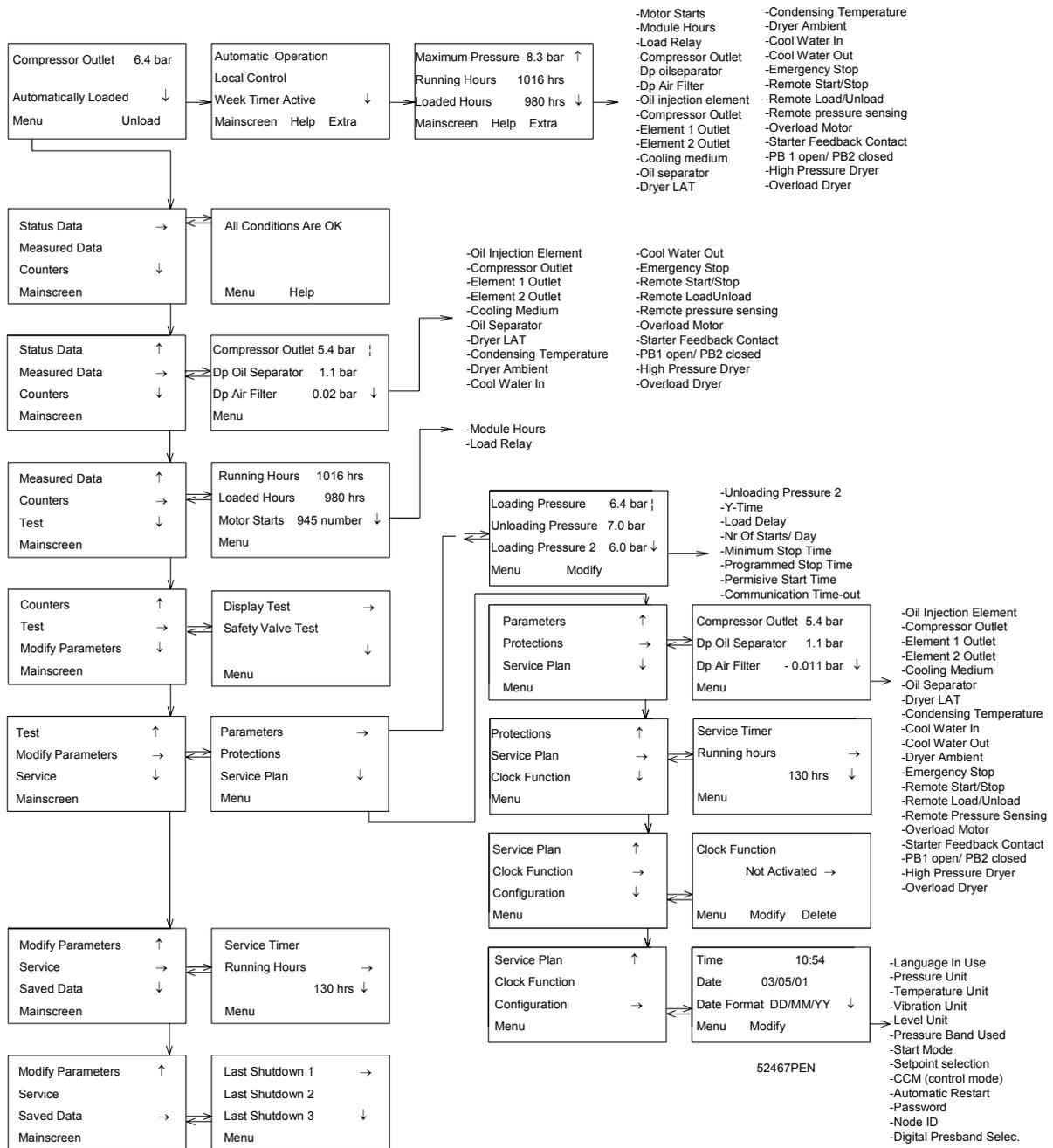
Fig. 4.2 Menu flow, GA90/315 watercooled
